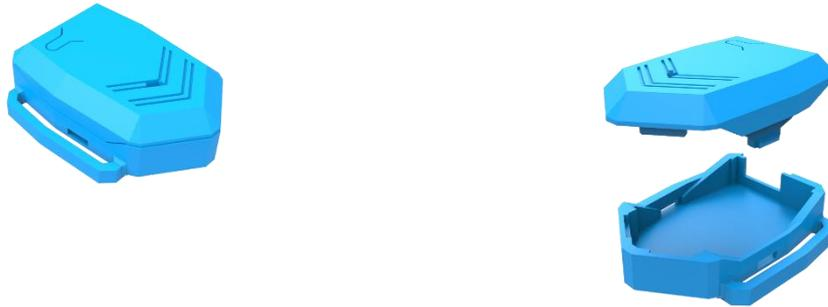
**FIG. 38 - Development of IMU case 3D model**
