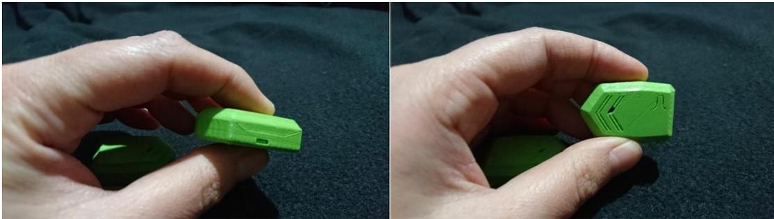
**FIG. 39 - Development of IMU case 3D printed model**
